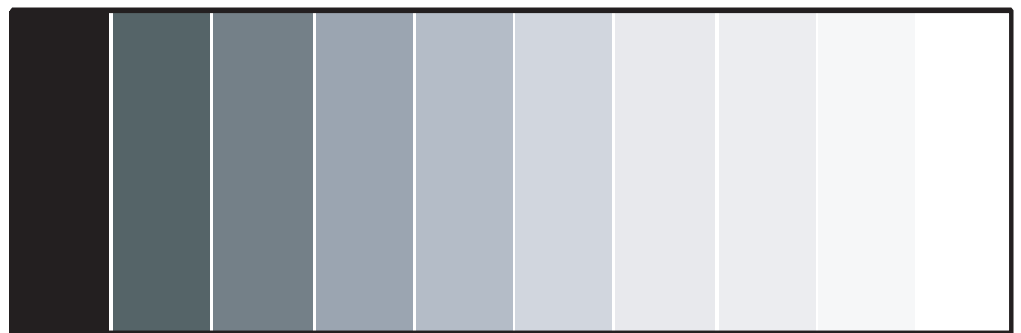
Figure 4-4. Typical Gray Bar Pattern for Adjusting Contrast
